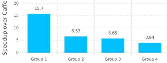
**Figure 15:** Breakdown of speedup for the first four groups of Convolution+ReLU+Pooling layers of VGG.
